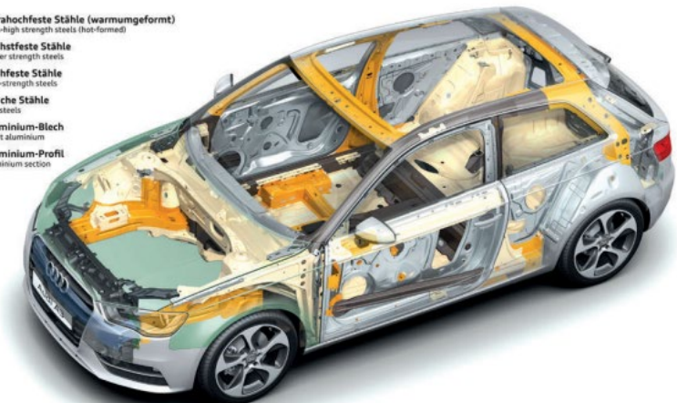
Audi A3 Karosseriematerialien Materials in the body structure 04/12
